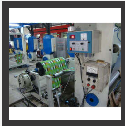
Web Tension Control System
