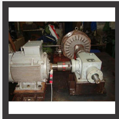
Bevel Gearbox Test Rig
