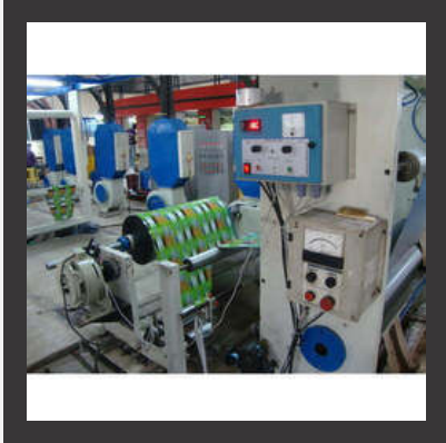
Web Tension Control System
