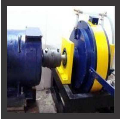
Electric Motor Test Rig
